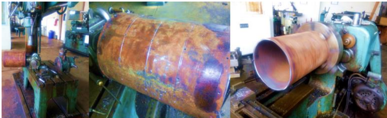
a) Drilling on radial drill b) Indexing of fastening holes c) Facing on lathe machine
