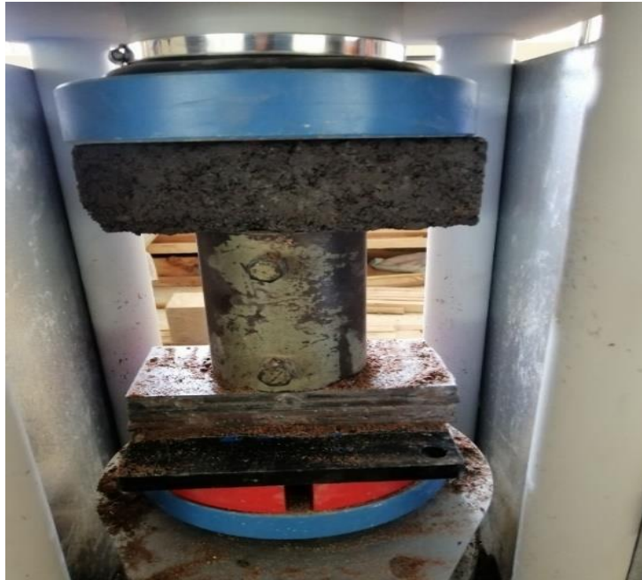
Figure 4: Compressive strength test.
