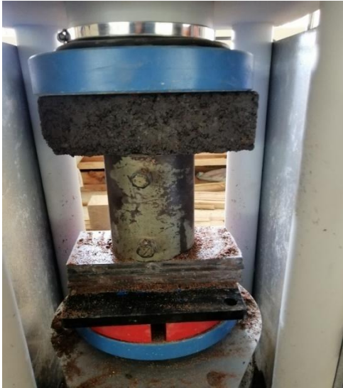
Figure 3: Compressive strength test.
