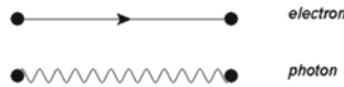
Fig. W.6 Electron propagator S_F(p) and photon propagator D_F^{\mu\nu}(k) in Feynman diagrams
