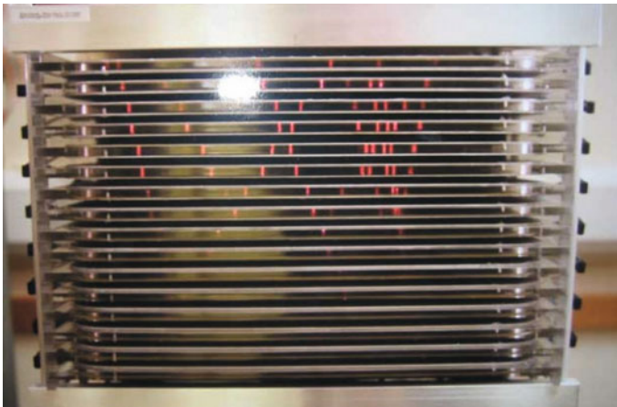
Fig. 4.18 The spark chamber built by LIP (Laboratório de Instrumentação e Partículas, Portugal) for educational purposes records a cosmic ray shower
