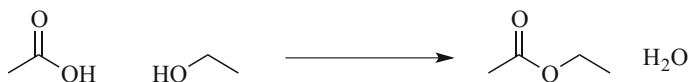
Fig. 3.18 The formation of an ester via a condensation reaction. Note the formation of water as one of the products
