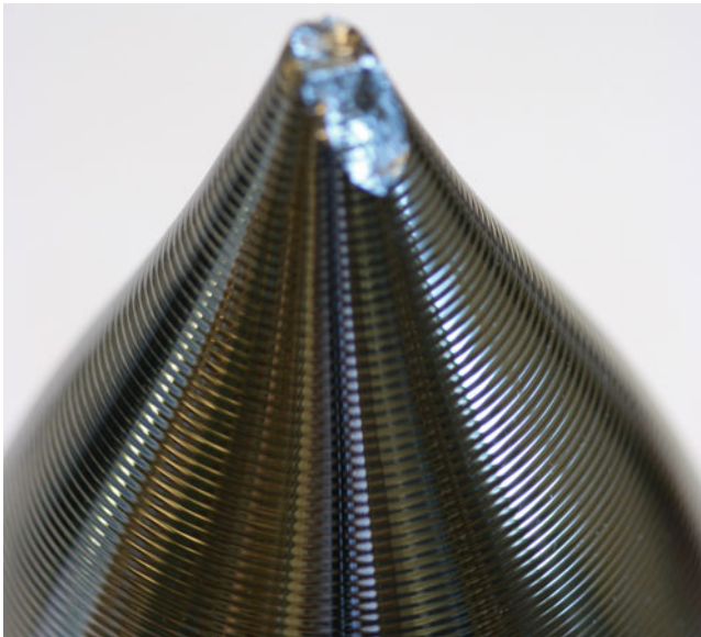
FIGURE 29.5. Growth rings on crystal surface: top section of Si crystal after removing seed.
