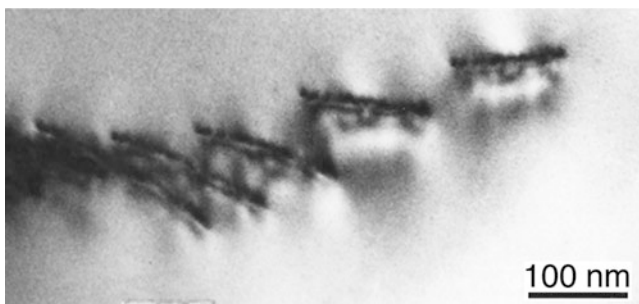
FIGURE 12.8. Diffraction contrast from dislocations in \text{Al}_2\text{O}_3 .
