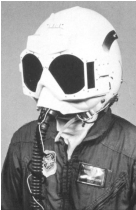
FIGURE 1.3. Pilot wearing the flash-blindness goggles (in the “off” position).
