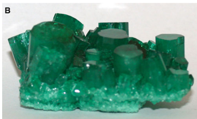
FIGURE 29.15. Flux growth of emerald. (A) Schematic. (B) Emeralds.
