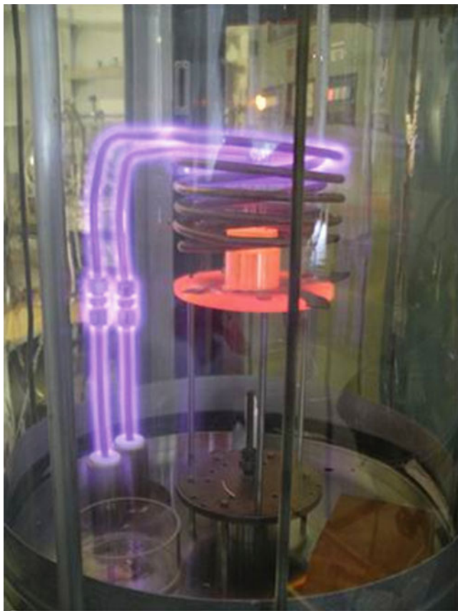
FIGURE 9.6. Induction furnace. The sample is mounted within the coils, which are usually water-cooled copper.
