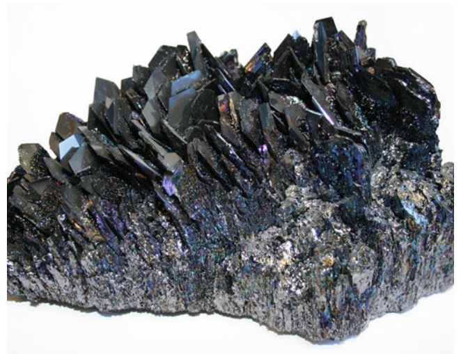
FIGURE 19.7. SiC produced by the Acheson process.
