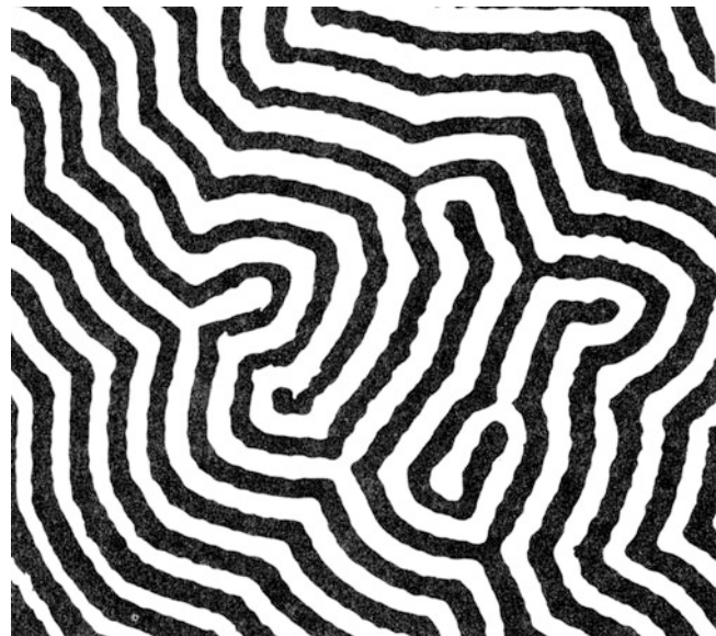
FIGURE 33.19. Domain pattern in a YIG thin film revealed by the Faraday effect.
