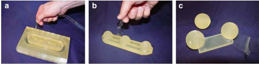
Fig. 8.2 Support material removal for three golf balls made using a Solidimension machine, showing: (a) the balls still encased in a central region, being separated from the larger block of bonded material; (b) the support material is glued in an accordion-like manner so that the excess material can be pulled out easily as a continuous piece; and (c) the balls after complete removal of excess support material (courtesy 3D Systems)
