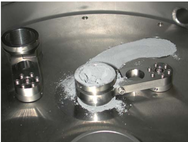
Fig. 5.11 3D Micromac Powder Feed System. In this picture, only one of the powder feeders (located over the build cylinder) is filled with powder (courtesy Laserinstitut Mittelsachsen e.V.)
