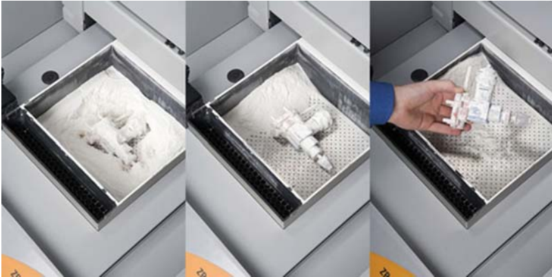
Fig. 16.1 Automated powder removal using vibratory and vacuum assist in a ZCorp 450 machine. (Courtesy Z Corporation)
