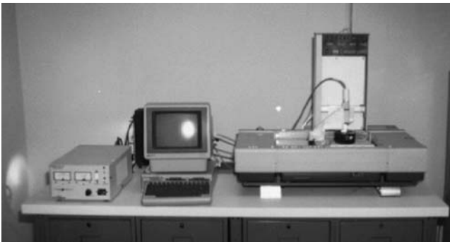
Fig. 2.7 The first AM technology from Hull, who founded 3D systems (photo courtesy of 3D Systems)
