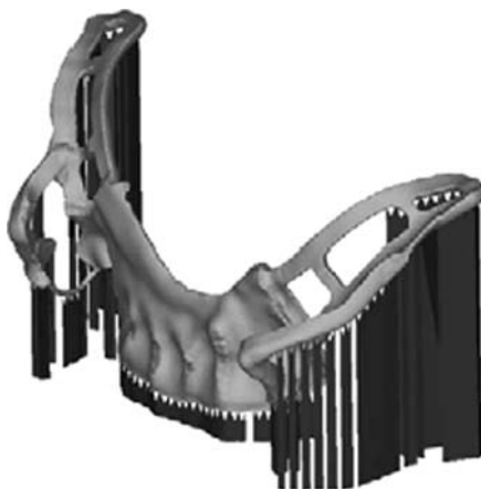
Fig. 16.5 SLM dental framework (© Emerald Group Publishing Limited) [1]
