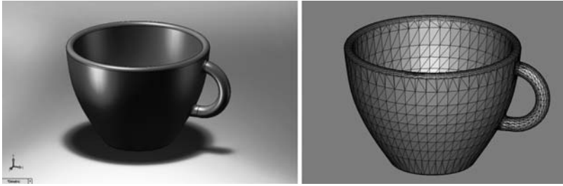
Fig. 2.2 A CAD model on the left converted into STL format on the right
