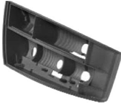
Fig. 17.7 A component made using Bluestone material. Note in particular the opacity of this SLA material, which in reality is a light blue color (image courtesy of 3D Systems)
