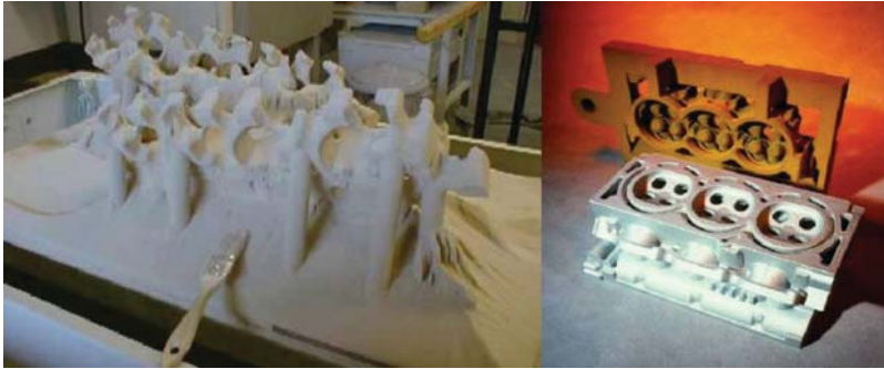
Fig. 16.12 Sand casting pattern for a cylinder head of a V6, 24-valve car engine ( left ) during loose powder removal and ( right ) pattern prepared for casting alongside a finished casting. (Joint project between CAD/CAM Becker GmbH and VAW Südalumin GmbH, made on an EOSINT S laser-sintering machine, courtesy EOS)
