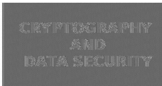
Fig. 5.3 Image and encrypted image using AES with 256-bit key in ECB mode
