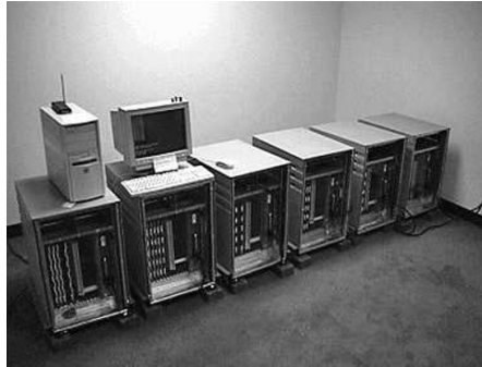
Fig. 3.15 Deep Crack — the hardware exhaustive key-search machine that broke DES in 1998 (reproduced with permission from Paul Kocher)
