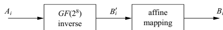
Fig. 4.4 The two operations within the AES S-Box which computes the function B_i = S(A_i)
