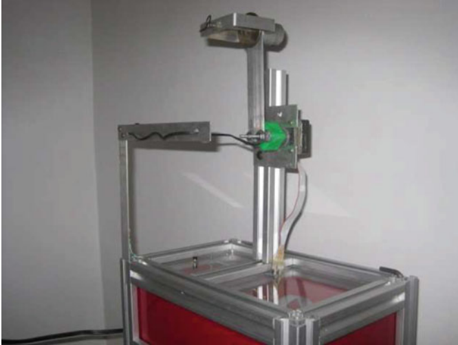
Fig. 16.14 The inertia wheel pendulum balancing at the inverted unstable configuration
