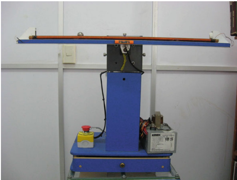
Fig. 14.18 Ball and beam system prototype that has been built
