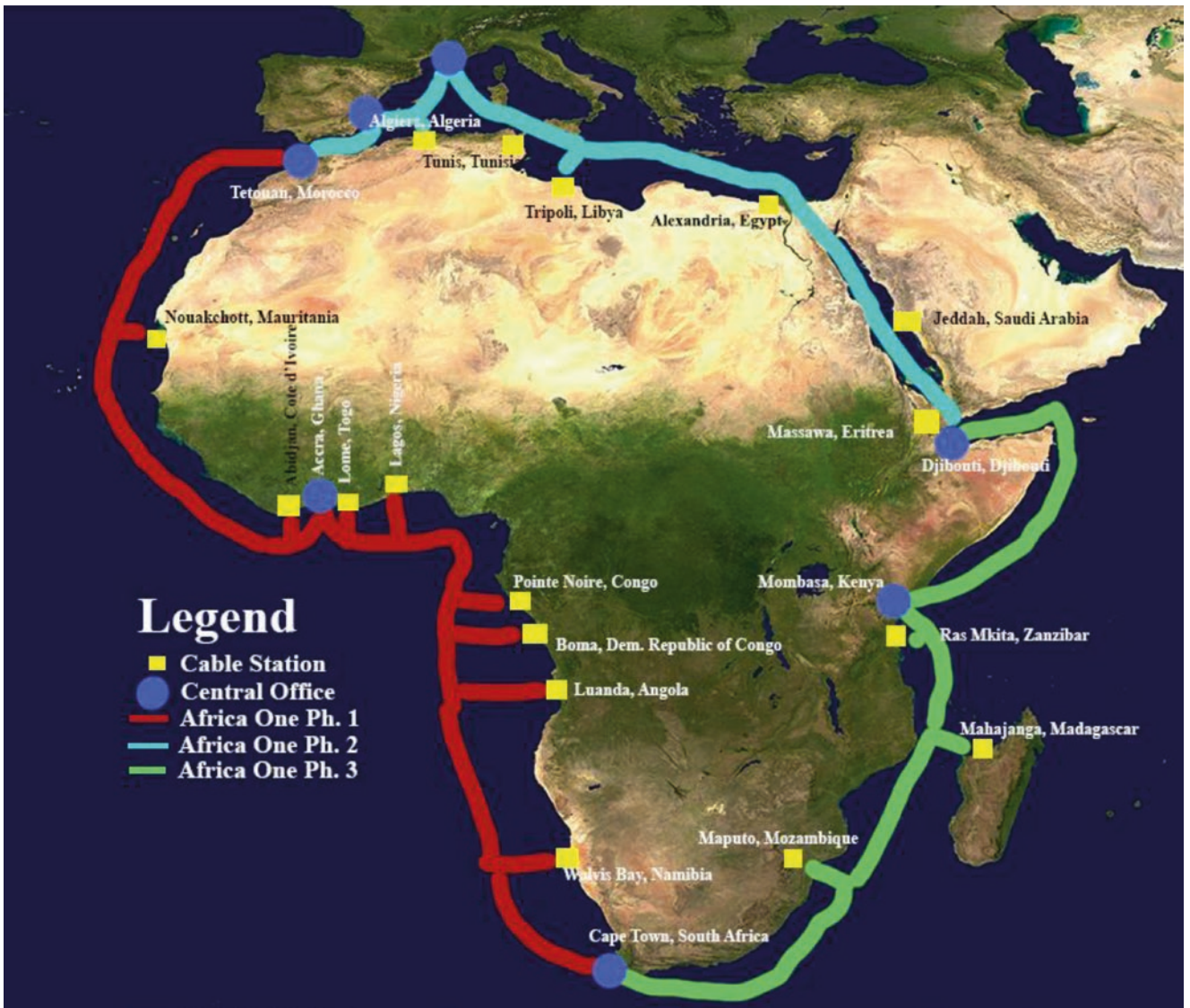
Fig. 12.8 Distribution model #2: The Bus or the Ring – Fiber network ring around Africa
