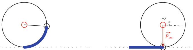
Fig. 15.13 Illustration of rolling condition: The point P is at a position \mathbf{p}_{cm} = -R \mathbf{j} relative to the center of mass
