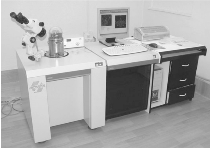
Fig. 7.13 Photograph of a JSPM-5200 scanning probe microscope
