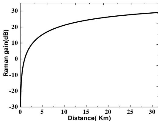
Fig 3 Attainment of a 30dB Raman gain over the total fibre length
