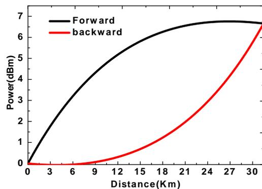
Fig 6 illustrates the Raman gain evolution over the total fibre length for forward and backward pumping configurations.
