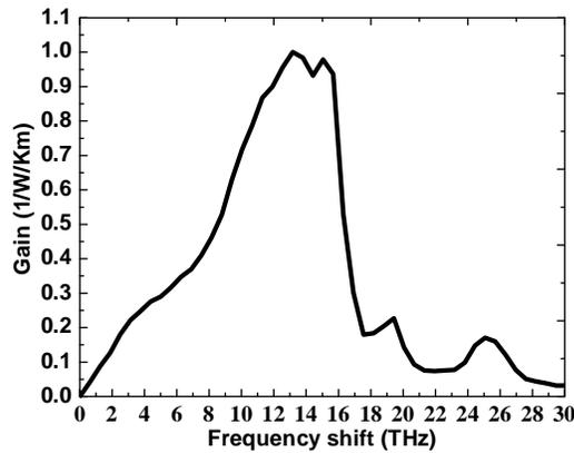
Fig 2 shows the normalized Raman gain profile
