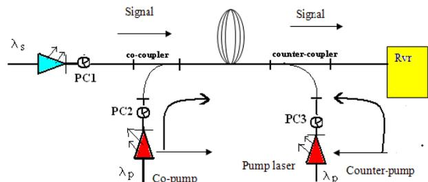
Fig 1 shows the design of a Raman amplifier
