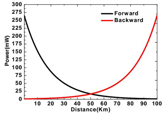
Fig 4 illustrates how pump power evolves over length for different pumping schemes (co- and counter- propagation)
