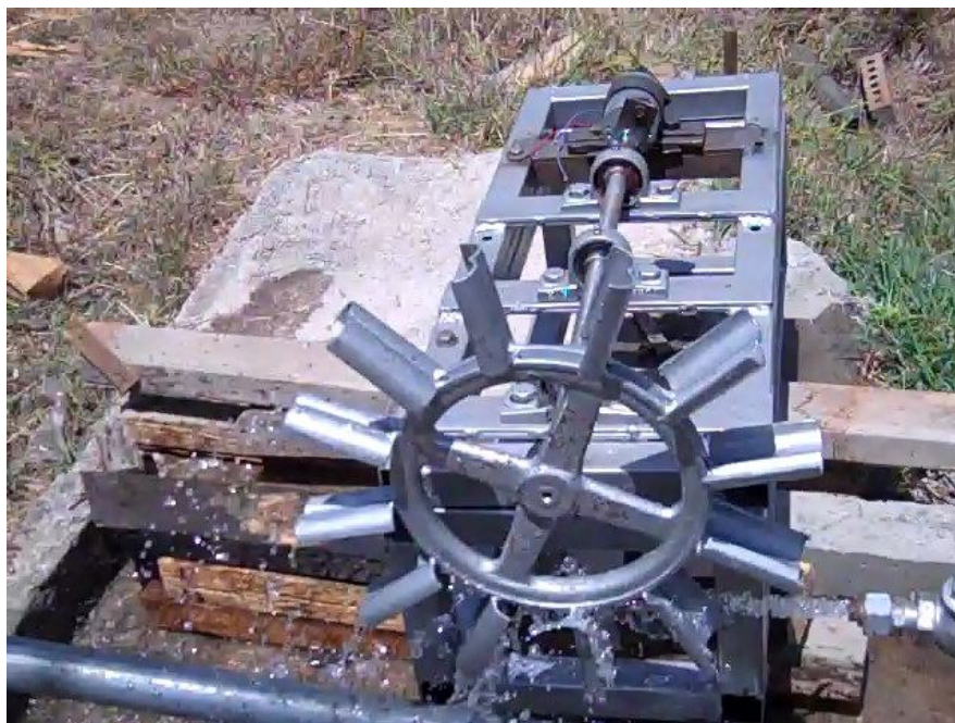
Figure 9: The fabricated pelton wheel turbine
