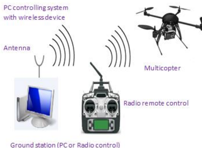
Figure 3. Basic and simple multicopter control system
