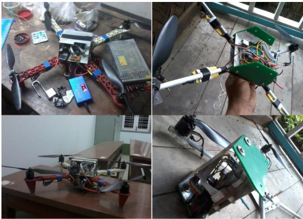
FCU assembled on the homemade aluminium and DJI frame
